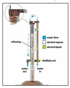
The saddles in the column provide a large surface area to maximise the contact between the liquid and vapour flows in the column, which accelerate the refluxing action.
