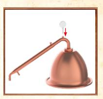
2 Insert the thermometer probe into the hole at the top of the column.
