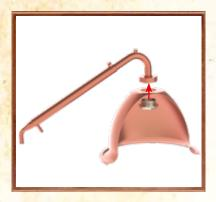
1 • Attach the copper condenser arm to the copper dome by removing the nut and O ring from the base of the condenser. Sit the condenser on the dome and screw the nut and O ring back into the condenser (check the lid isn't spinning anymore) to firmly attach the dome to the condenser.
