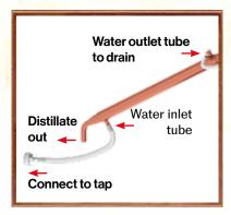
4 Briefly turn on the cooling water supply to ensure there are no leaks in the system. Check again that the water goes in at the end where the distillate comes out and that the water comes out closest to the top of the lyne arm (at the end near the thermometer probe).
